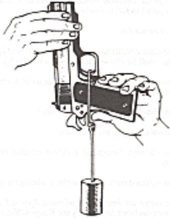
Fig. 5 - Correct Method of Weighing Triggers
